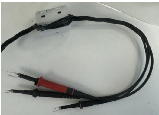
Figure 32. Filtering Common Mode Gate to Source Noise with Ferrite Core on Twisted Wires
