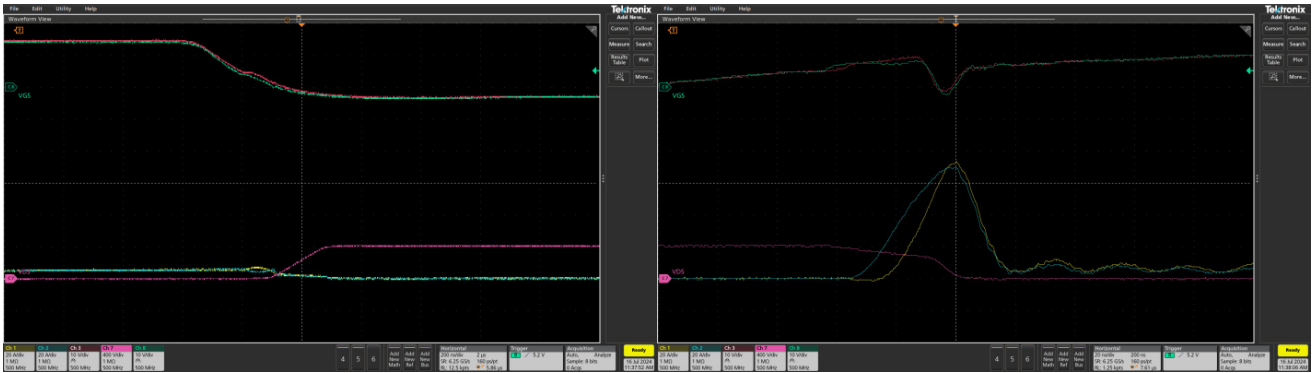
Figure 25. Ls Unbalance with Ferrite Bead on Both Gate and Kelvin-source (DC link 400 V, I_D = 6 A)
